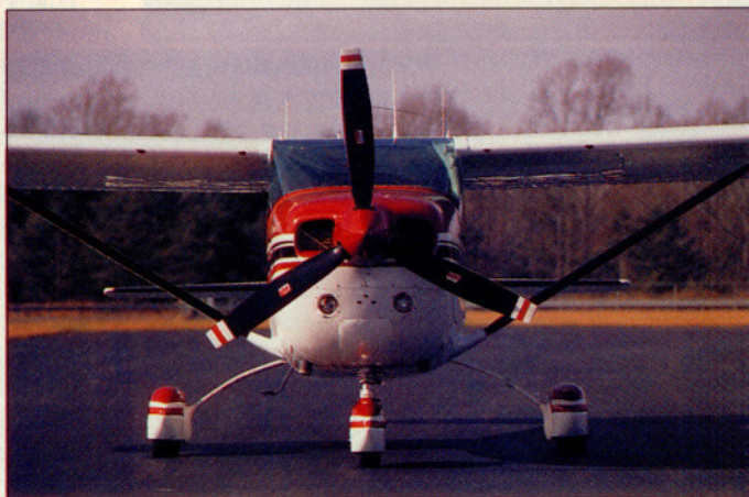
The 550 conversion includes either a Hartzell or McCauley (above) three-bladed propeller. A new tach and fuel flow gauge are also included.
